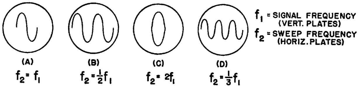
FIGURE 2-4 SIGNAL VS. SWEEP RELATIONS AS VIEWED ON OSCILLOSCOPE SCREEN
