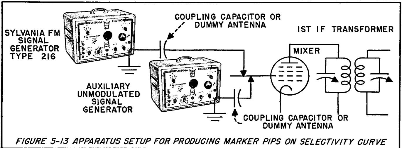
fier has been correctly aligned with an FM signal generator connected to the mixer control grid, apply a signal at the same time to the same grid from a second, unmodulated signal generator set to the intermediate frequency (see Figure 5-13).
