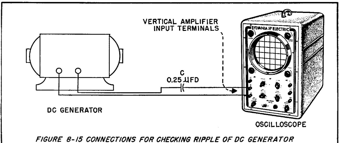
FIGURE 8-15 CONNECTIONS FOR CHECKING RIPPLE OF DC GENERATOR
