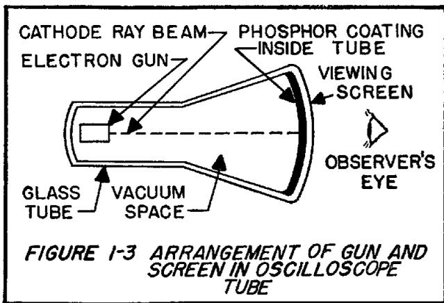
chemical, it will glow at the point where the electron beam strikes it. This will produce a small, bright dot, at that point, but elsewhere the fluorescent surface will not be affected. In the modern oscilloscope tube employed by radio engineers and servicemen, emission of electrons is effected by heating a cathode, rather than as shown in Figures 1-1 and 1-2.
