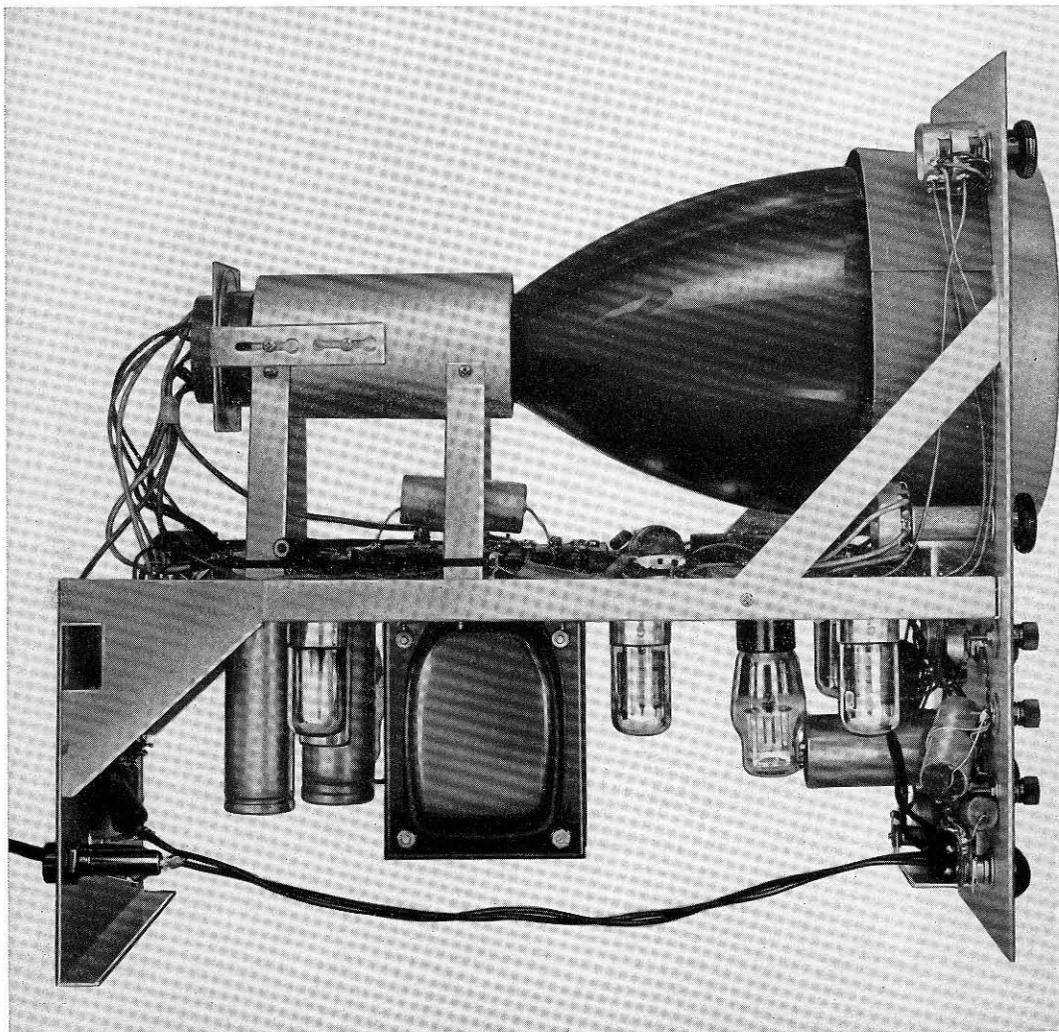
*FIGURE 3-7 Inside view of Sylvania Seven-Inch Oscilloscope Type 132. Construction is similar to that of Type 131 three-inch instrument except that higher voltage components and larger tubes are necessary. Circuit is also more complicated. (See Figure 3-4).*
