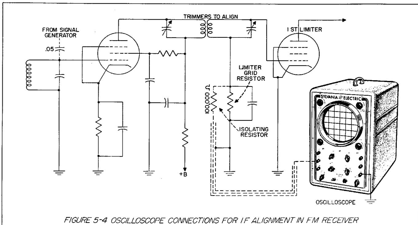
FIGURE 5-4 OSCILLOSCOPE CONNECTIONS FOR IF ALIGNMENT IN FM RECEIVER
