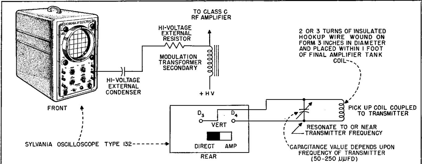
FIGURE 7-2 OSCILLOSCOPE CONNECTIONS TO TRANSMITTER FOR TRAPEZOIDAL MODULATION PATTERNS
