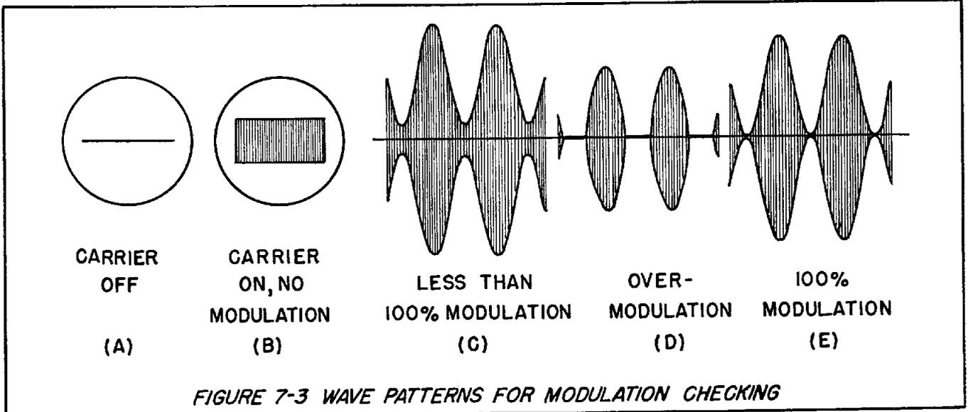
FIGURE 7-3 WAVE PATTERNS FOR MODULATION CHECKING
