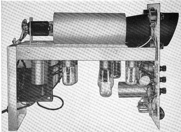
*FIGURE 3-6 Inside view of Sylvania Three-Inch Oscilloscope Type 131. Note large metal shield around neck of tube. Tubes and other circuit components are mounted below 3AP1 tube. Power transformer (lower left) is mounted as far as possible from tube to prevent hum modulation of electron beam.*
