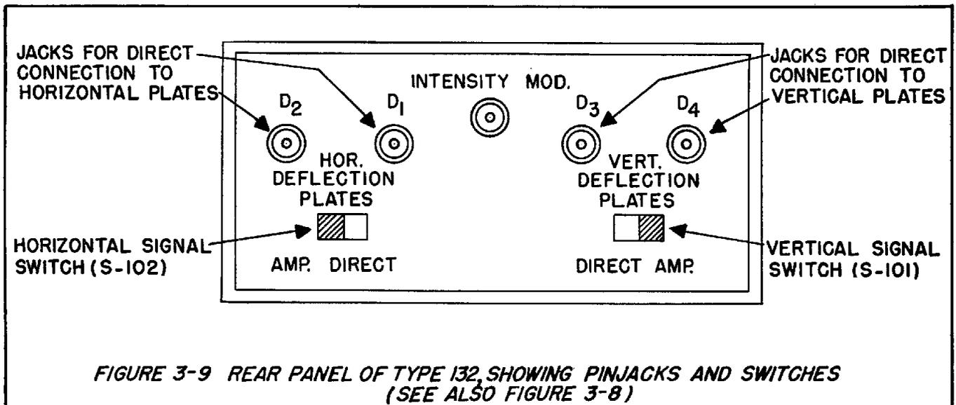
FIGURE 3-9 REAR PANEL OF TYPE 132, SHOWING PINJACKS AND SWITCHES (SEE ALSO FIGURE 3-8)
