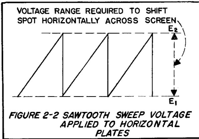
then falls quickly back to level  $E_1$ . The sharp drop from  $E_2$  to  $E_1$  must occur in a small fraction of the time required for the completion of one cycle of the signal voltage applied to the vertical plates.
