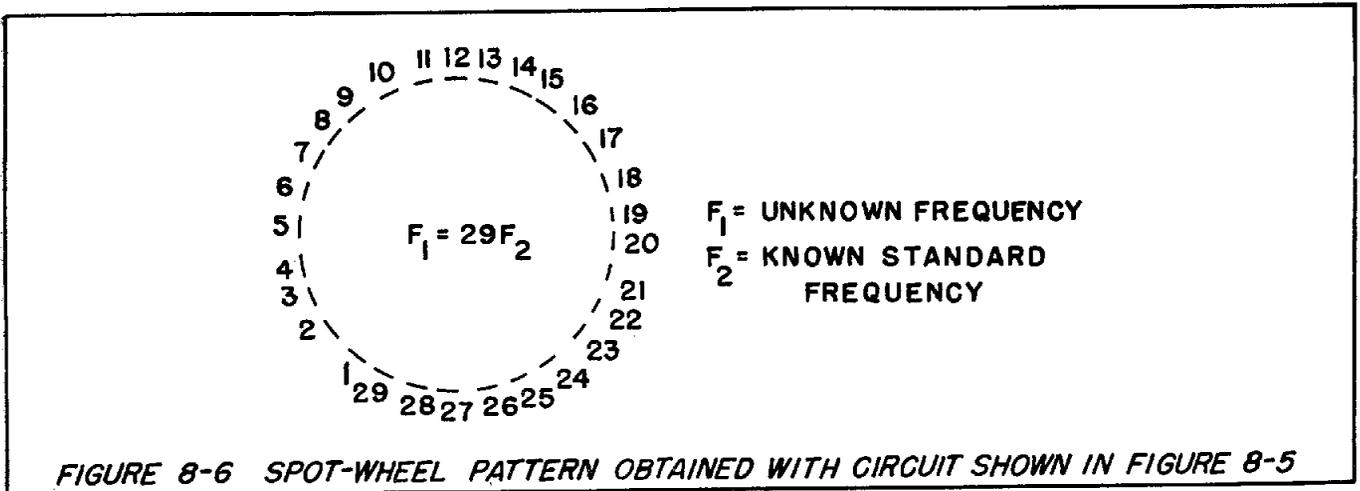
the fine frequency control of the oscilloscope for each setting of the coarse frequency control.
