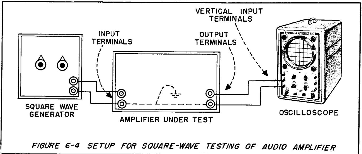
generator output terminals to input terminals of amplifier under test.
