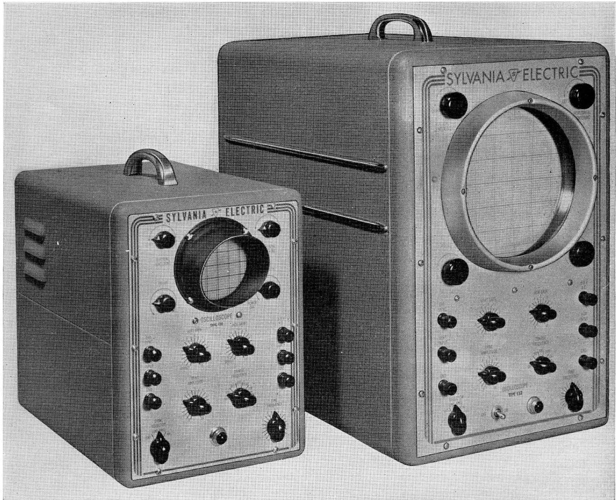
*On the left is the Sylvania Three-Inch Oscilloscope Type 131 and on the right, the Sylvania Seven-Inch Oscilloscope Type 132. Use of these instruments in servicing AM and FM radio receivers and many other applications is described in detail in this book.*
