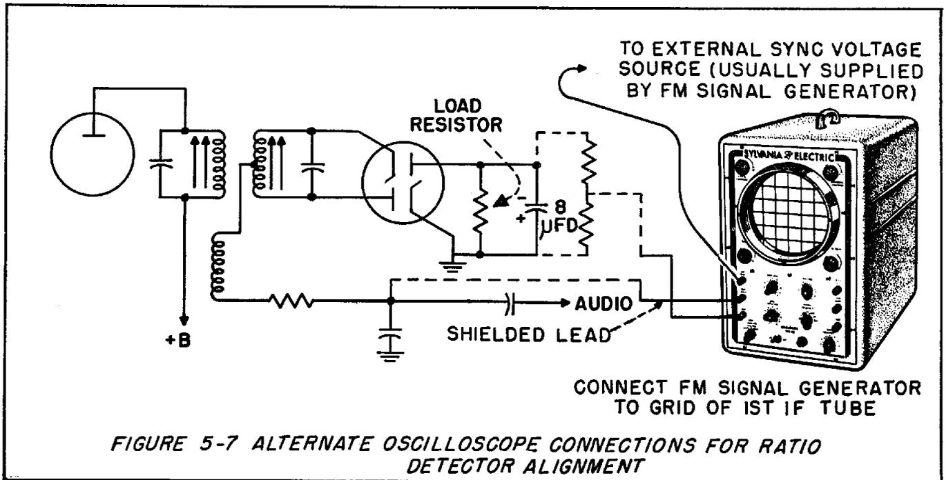
FIGURE 5-7 ALTERNATE OSCILLOSCOPE CONNECTIONS FOR RATIO DETECTOR ALIGNMENT
