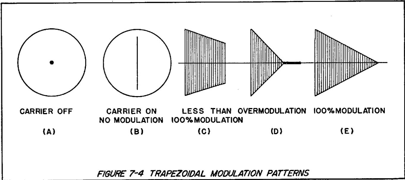
FIGURE 7-4 TRAPEZOIDAL MODULATION PATTERNS
