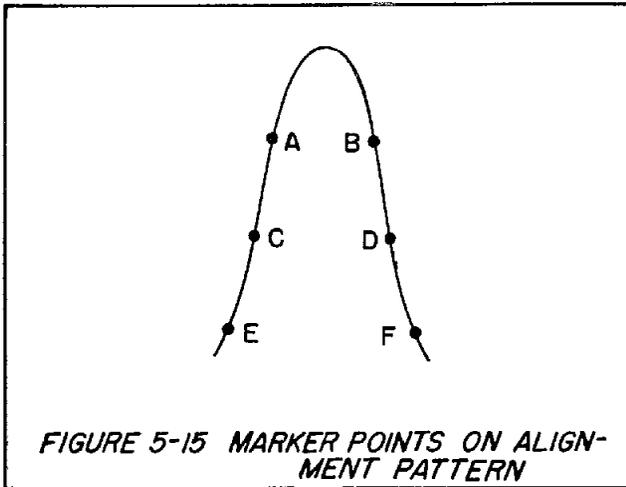
of the pulse generator. Thus, if the repetition rate is 10,000 cycles, the points will be 10 kc apart along the curve.
