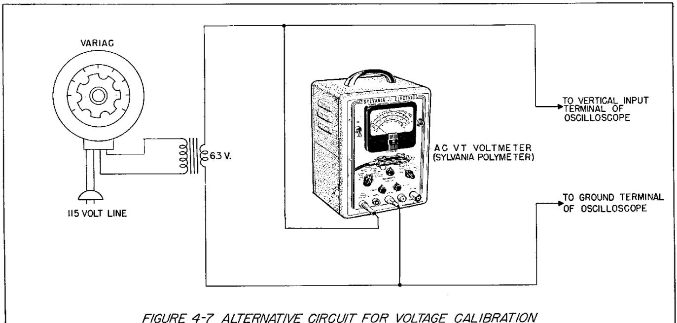
FIGURE 4-7 ALTERNATIVE CIRCUIT FOR VOLTAGE CALIBRATION
