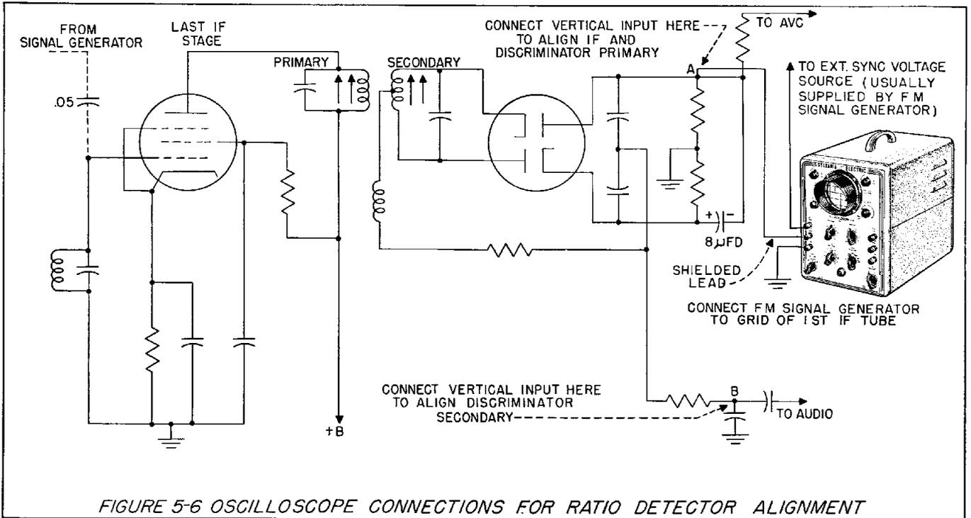
FIGURE 5-6 OSCILLOSCOPE CONNECTIONS FOR RATIO DETECTOR ALIGNMENT
