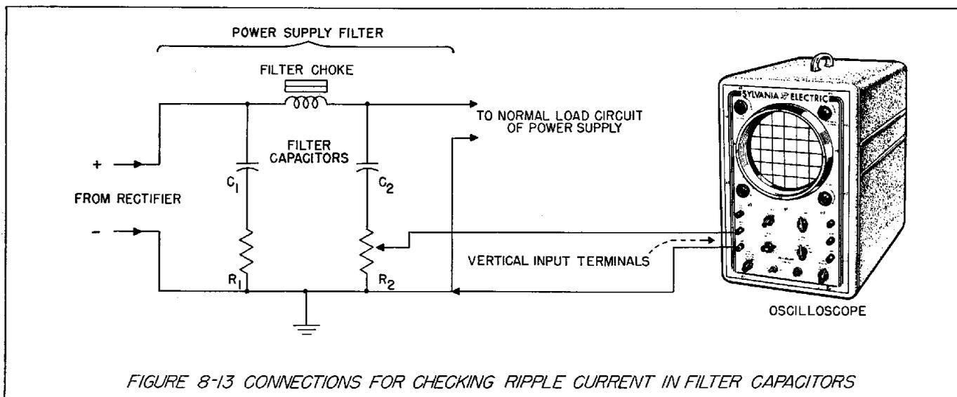
FIGURE 8-13 CONNECTIONS FOR CHECKING RIPPLE CURRENT IN FILTER CAPACITORS
