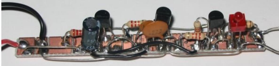
The transmitter is built on a small length of PC board, cut into lands with a file. The photo clearly shows how all the components are mounted and how the board is fitted into a toothbrush holder. The flashing LED shows the unit is ON and serves to control the beep-beep-beep of the circuit. The flashing LED is not an ordinary LED.
