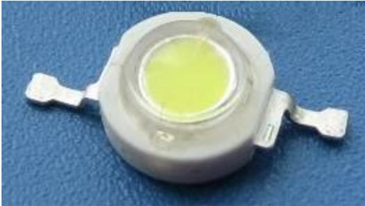
The circuit will not drive two LEDs in series - it runs out of voltage (and current) when the voltage across the load is 7v. It oscillates at approx 200kHz. Build both the 20 LED and 1 watt LED version and compare the brightness and effectiveness. The photo of the 1 watt LED on the left must be heatsinked to prevent the LED overheating. The photo on the circuit diagram shows the LED mounted on a heatsink and the connecting wires.
