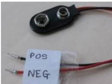
The battery snap plugs into the pins on the 5v regulator board with the red lead going to the negative output of the board as the battery snap is now DELIVERING voltage to the circuit you are powering.
