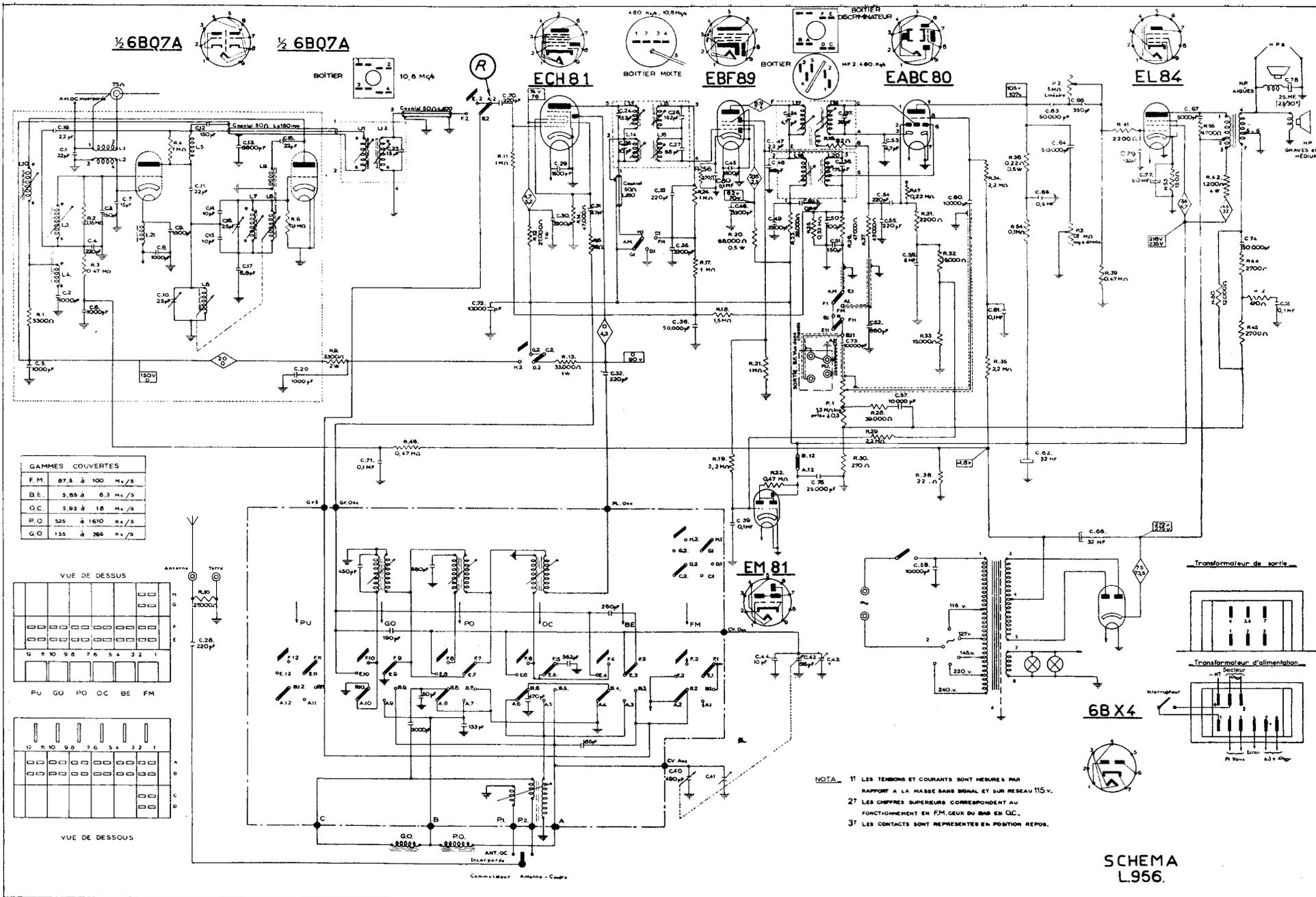
NOTA 1) LES TENSIONS ET COURANTS SONT MESURES PAR RAPPORT A LA MASSE SANS SIGNAL ET SUR RESEAU 115V.
